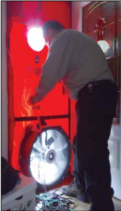
An energy audit of your home may include a blower door test like this one to determine how much air is filtering out of your house.
